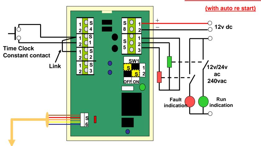
The above example is to be used for volt free time clock control constant contact
