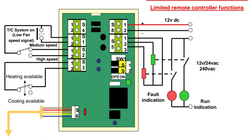
The above example is to be used for volt free time clock control constant contact, a remote Heat / cool input is required, and a remote Fan speed input.
