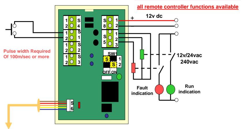
The above example is to be used for volt free time clock control pulsed contact
