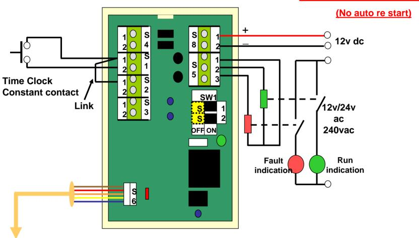
The above example is to be used for volt free time clock control constant contact
