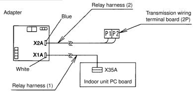
Make connections as shown above, using the attached relay harnesses (1) and (2).
