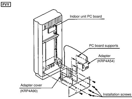
Note: optional adaptor box is required to install the adapter
