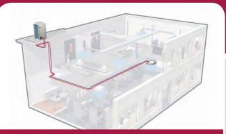
**PIPING LENGTH INDOOR – OUTDOOR:** Maximum piping length outdoor-all indoors: up to 165m Maximum installation height difference outdoor-indoor: up to 30m
