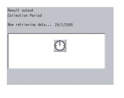
In case the power proportional distribution report is missing, the display indicates the list of missing data (day / month / year / time). The list indicates up to a maximum of 100 cases. If the missing data exceed 100 cases, the list indicates only the first 100 cases. If OK button is pressed, the display indicates the power proportional distribution report.
