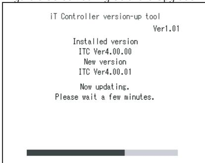
Figure 7 Screen during Software Upgrade
