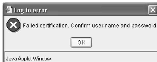
If the Administrator attempts to log into the web interface without closing the system menu on the intelligent Touch Controller console, the error message ((2) in the figure) appears. In this case close the system menu, and log into it again.
