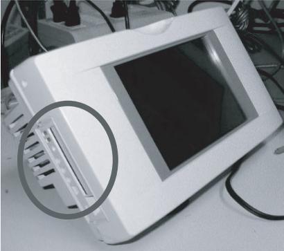
Figure 2 Reset Switch Position
