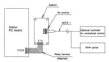
NOTE 1. Wiring specifications . . . Use a 0.75 – 1.25 mm² sheathed vinyl cord or cable (2 wire).
