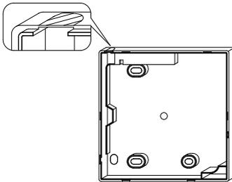
Cut off thin area (hatched area) with nippers or the like, and then remove burr with a file or the like.
