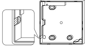
Cut off thin area (hatched area) with nippers or the like, and then remove burr with a file or the like.
