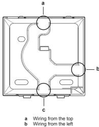
c Wiring from the bottom
