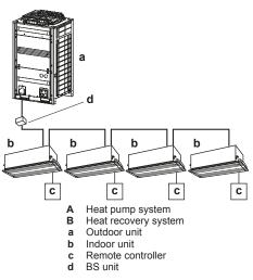
When multiple indoor units are connected to an outdoor unit, one of these units (or a group of indoor units, in case of group control) needs to be set as Cooling/Heating master. The other units/groups then become Cooling/Heating slaves, and are restricted in their operation by the master (e.g. one outdoor unit does not allow for one indoor unit to run in Cooling operation while another runs in Heating operation).
