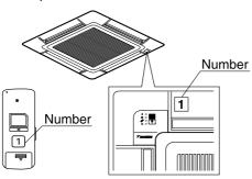
Operate the indoor unit with the remote controller of the same number.
