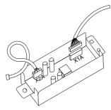
After connecting, use the attached clamp to fix the two harnesses to the transmitter board box.
