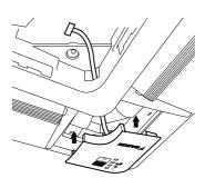
Hook the harness from the receiver on the upper part of the panel temporary suspension of the decoration panel. Be sure to push the harness to the groove.
