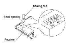
After completing setting, seal off the opening of the address switch and the MAIN/SUB switch with the attached sealing pad.
