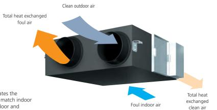
The Daikin heat recovery ventilation system modulates the temperature and humidity of incoming fresh air to match indoor conditions. A balance is thus achieved between indoor and outdoor ambients, enabling the cooling or heating load placed on the air conditioning system to be reduced significantly. HRV units can be controlled individually or integral with the air conditioning system (Daikin VRV® or Sky Air series).
