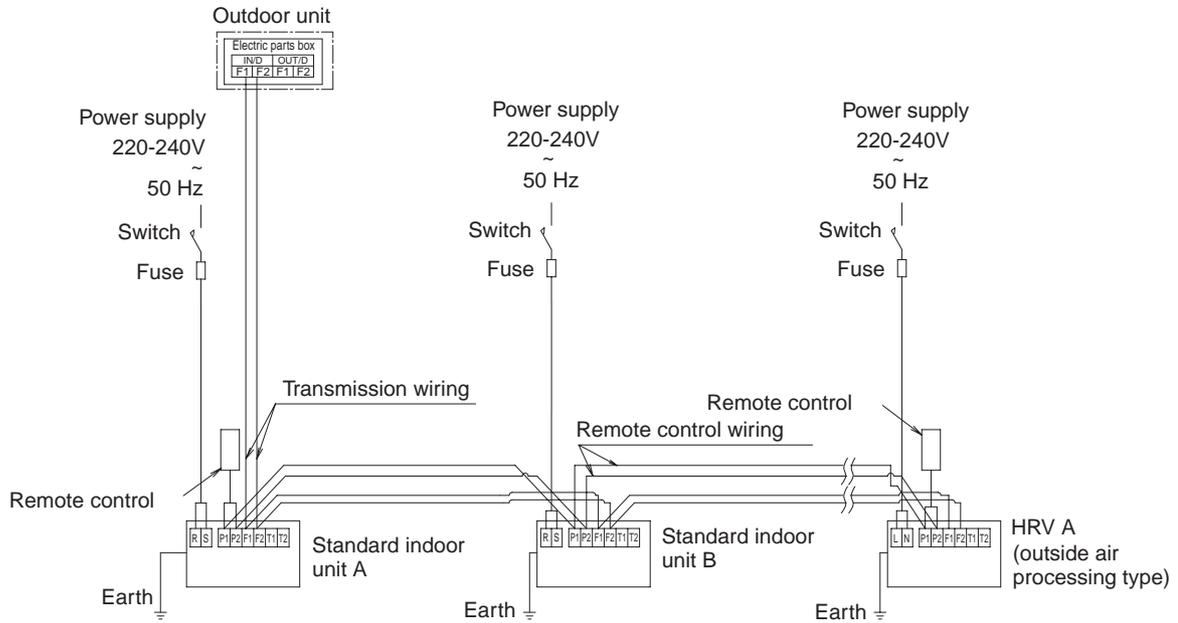
**(Independent system (connected only with a HRV unit in a single refrigerant circuit))**
