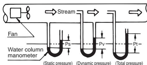
“Static pressure (Ps)” is a pressure needed for overcoming the resistance of the duct when conveying air.
