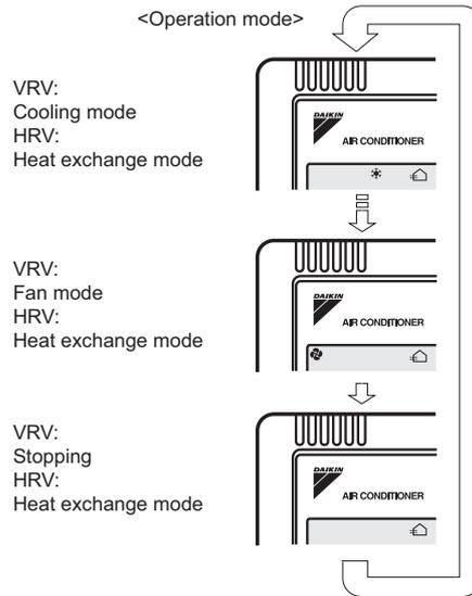
When air conditioner and HRV unit are connected via duct
