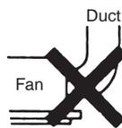
Bending the duct near the shutter frame may not permit the shutter to open completely. To avoid this, there should be a distance of minimum 150 mm between the bend and shutter.
