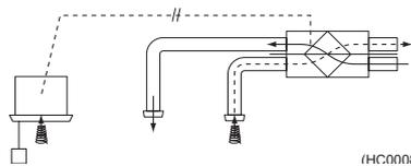
The HRV unit cannot be operated independently when the air conditioner is connected to the HRV unit via a duct. When using the HRV unit, set the air conditioner to “fan” mode on weak fan strength.
