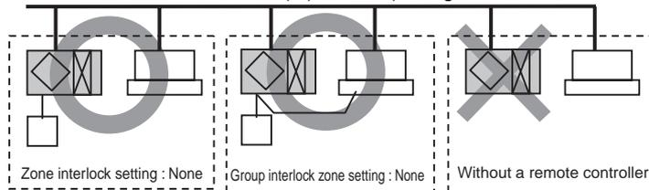
\* Alteration of set temperature and independent ventilation operation cannot be performed from a central device.
