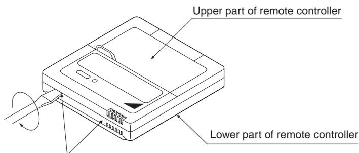
Insert the screwdriver here and gently work off the upper part of remote controller.
