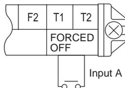
\* The equipment in Nighttime free cooling operation cannot be stopped forcibly with T1 or T2.
