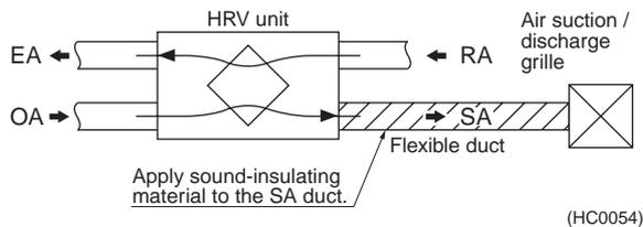
2. Operating sound can be reduced more effectively by applying sound-insulating material to a portion of the SA duct near the unit body than that near the air suction / discharge grille.
