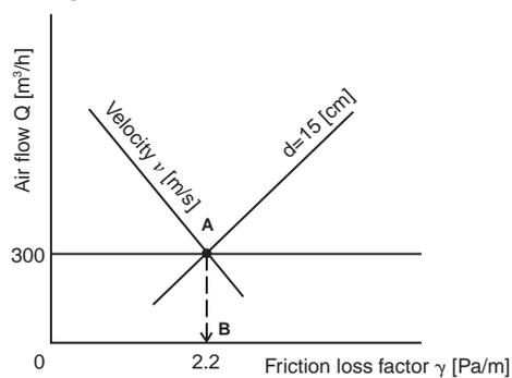
1. Find the intersection of the duct diameter  $d$  (15 cm) and air flow  $Q$  (300 m<sup>3</sup>/h) => Point **A**
