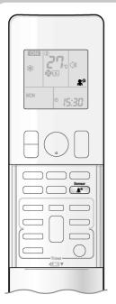
"INTELLIGENT EYE" is the infrared sensor which detects the human movement. If nobody in the room for more than 20 minutes, the operation automatically changes to energy saving operation.
