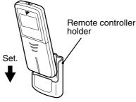
•To remove, pull it upwards.
