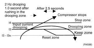
When a "stop current" continues for 2.5 seconds after rushing on the stop zone, the compressor operation stops.
