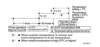
In case of FTK(X)S25-35E, FTK(X)S20-35D, FTK(X)S50-71F the temperature rises once.
