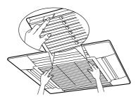
2. Detach the suction grille. Open the suction grille 45 degrees and lift it upward.
