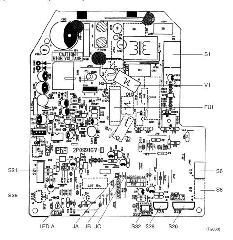
PCB(2): Signal Receiver PCB
