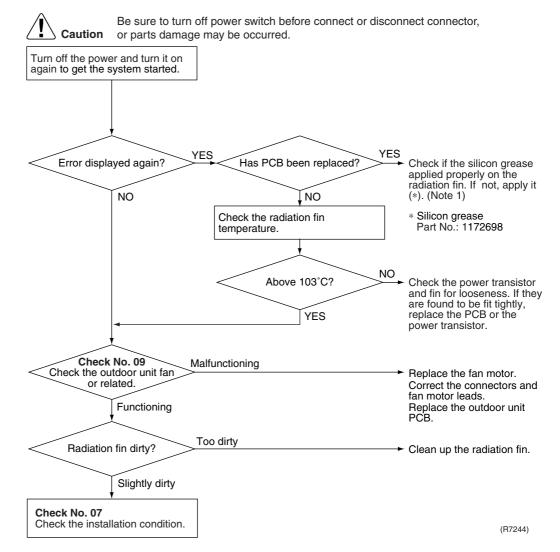
Note1: Refer to "1.3 Application of Silicon grease to a power transistor and a diode bridge" on P302.
