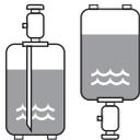
Charge the liquid refrigerant with the cylinder in up-side-down position.
