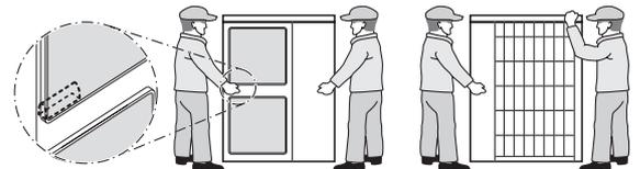
Place your hands on the corner instead of holding the suction inlet in the side of the casing, otherwise the casing could be deformed.
