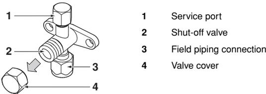
■ Since the side boards may be deformed if only a torque wrench is used when loosening or tightening flare nuts, always lock the stop valve with a wrench and then use a torque wrench. Do not place wrenches on the valve cover.
