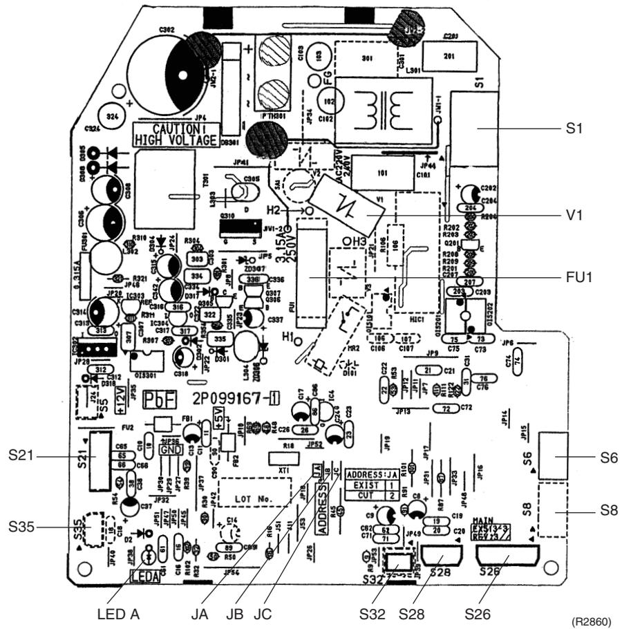
PCB(2): Signal Receiver PCB
