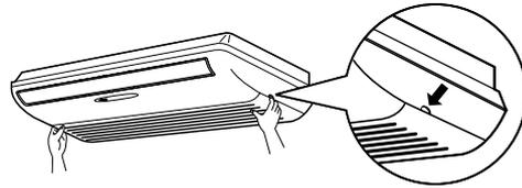
3. **Take off the air purifying filter, photocatalytic deodorizing filter.**
