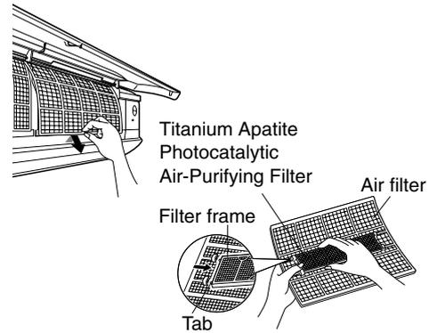
5. **Set the air filter and Titanium Apatite Photocatalytic Air-Purifying Filter as they were and close the front panel.**
