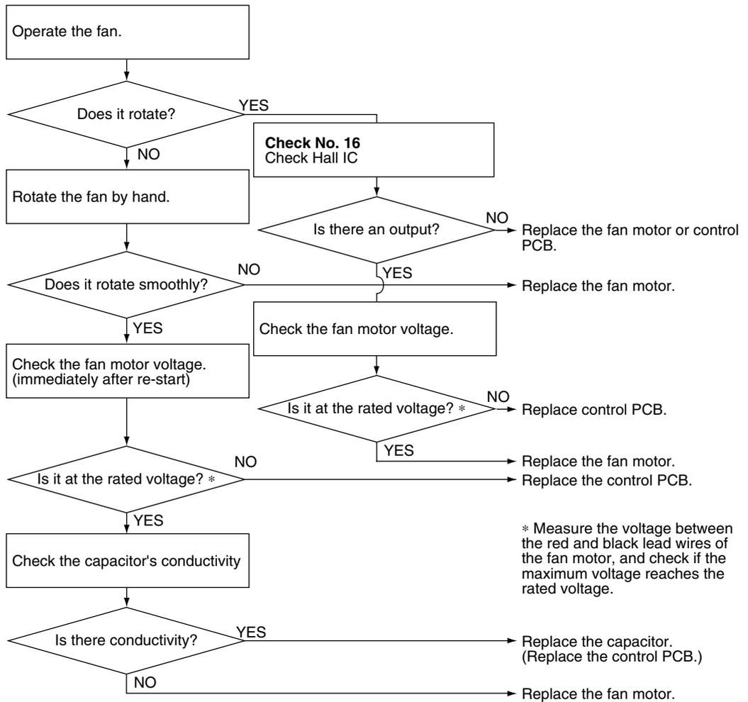
\* Measure the voltage between the red and black lead wires of the fan motor, and check if the maximum voltage reaches the rated voltage.
