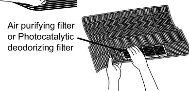
5. **Set the air filter, air purifying filter and photocatalytic deodorizing filter as they were and close the front panel.**
