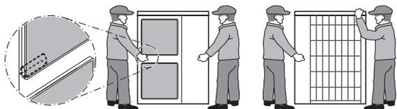
Place your hands on the corner instead of holding the suction inlet on the side of the casing, otherwise the casing could be deformed.
