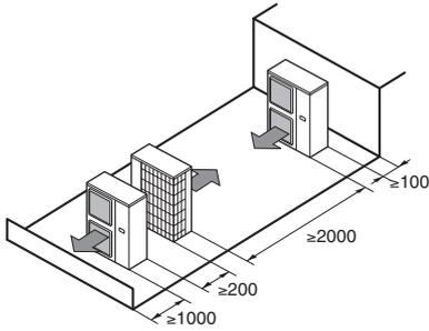
2. In case of installing multiple units (2 units or more) in lateral connection per row.
