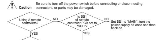
Set one remote controller to "MAIN"; turn the power supply off once and then back on.
