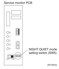
2. Install the removed jumper switch as described below. This jumper switch is needed later to disable this setting.
