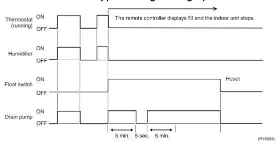
During heating operation, if the float switch is not reset even after the 5 minutes operation, 5 seconds stop, 5 minutes operation cycle ends, operation continues until the switch is reset.
