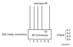
5. If the continuity is confirmed in the above step 3, the PCB is faulty.
