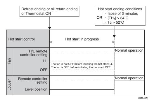
$\ensuremath{\mathsf{TH}}_2\ensuremath{\mathsf{:}}$  Temperature (°C) detected with the gas thermistor
