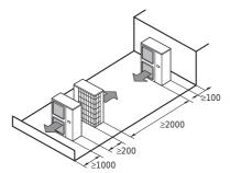
**2.** In case of installing multiple units (2 units or more) in lateral connection per row.
