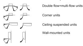
For the following conditions, a micro computer controls the air flow direction which may be different from the display.
