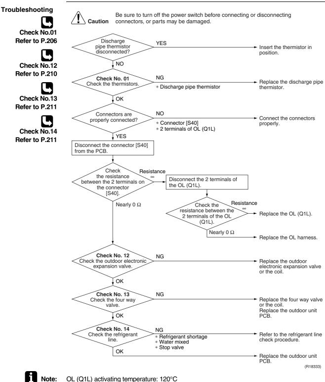
OL (Q1L) activating temperature: 120°C OL (Q1L) recovery temperature: 95°C
