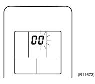
7. Press the [Temp]  $\blacktriangle$  or  $\checkmark$  button and change the number until you hear the long beep.
