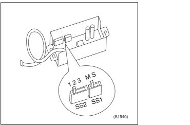
After completing setting, seal off the opening of the address setting switch (SS2) and the MAIN / SUB setting switch (SS1) with the attached sealing pad.
