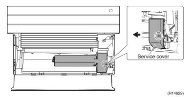
(3)Turn on the DIP switch [S2W-1] on the service PCB.
