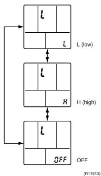
Press the [Mode] button for 5 seconds to exit from the brightness setting mode. (When the remote controller is left untouched for 60 seconds, it returns to the normal mode also.)
