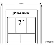
9. Press the [ON/OFF] button twice to return to the normal mode.
