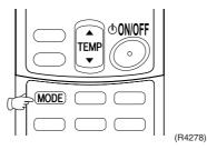
The display **7**<sup>-</sup> means the trial operation mode. (Refer to page 221 for trial operation.)
