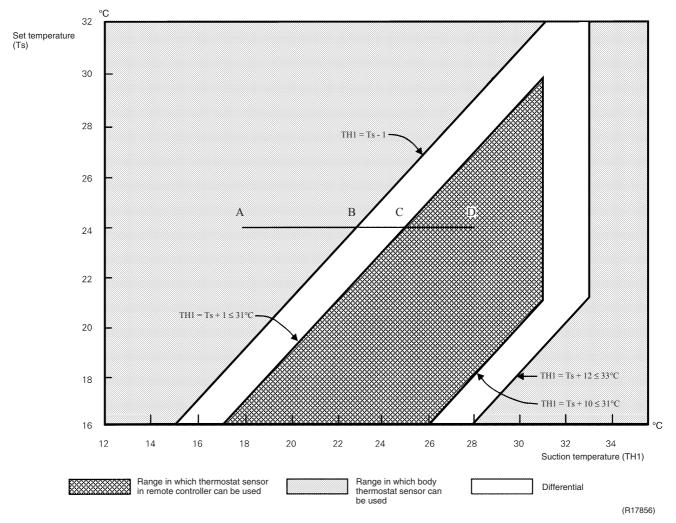
■ Assuming the set temperature in the figure above is 24°C, and the suction temperature has changed from 18°C to 28°C (A → D):
