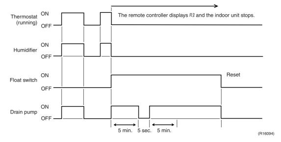
During heating operation, if the float switch is not reset even after the 5 minutes operation, 5 seconds stop, 5 minutes operation cycle ends, operation continues until the switch is reset.
