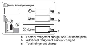
2 Fix the label on the inside of the outdoor unit. There is a dedicated place for it on the wiring diagram label.
