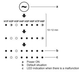
If the default situation is not displayed after 10~12 minutes, check the malfunction code on the indoor unit user interface. Solve the malfunction code accordingly. First, check the communication wiring.
