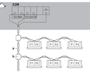
a Use the conductor of sheathed wire (2 wire) (no polarity)b Terminal board (field supply)
