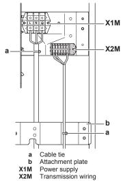
5 Route the wiring through the frame and connect it to it.
