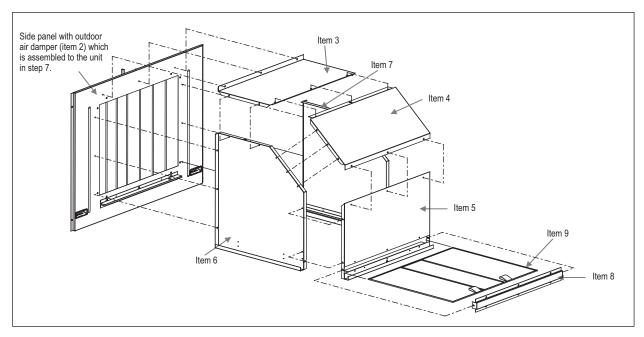
It is recommended to seal off all the joints and gaps with weather-proof sealant (such as silicone, field supplied item) in order to ensure a water-proof finishing on the rain hood.
