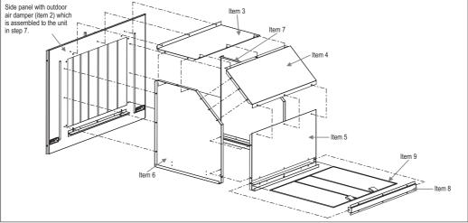
It is recommended to seal off all the joints and gaps with weather-proof sealant (such as silicone, field supplied item) in order to ensure a water-proof finishing on the rain hood.
