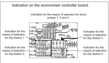
• There are two LEDs in economiser controller board, which are green LED and red LED. Green LED will blink when economiser controller board is powered-up. Red LED will blink when error(s) occur. Refer the table below for error codes and their meaning:
