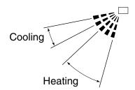
We recommend using the airflow in the position listed above when fixing the airflow direction.
