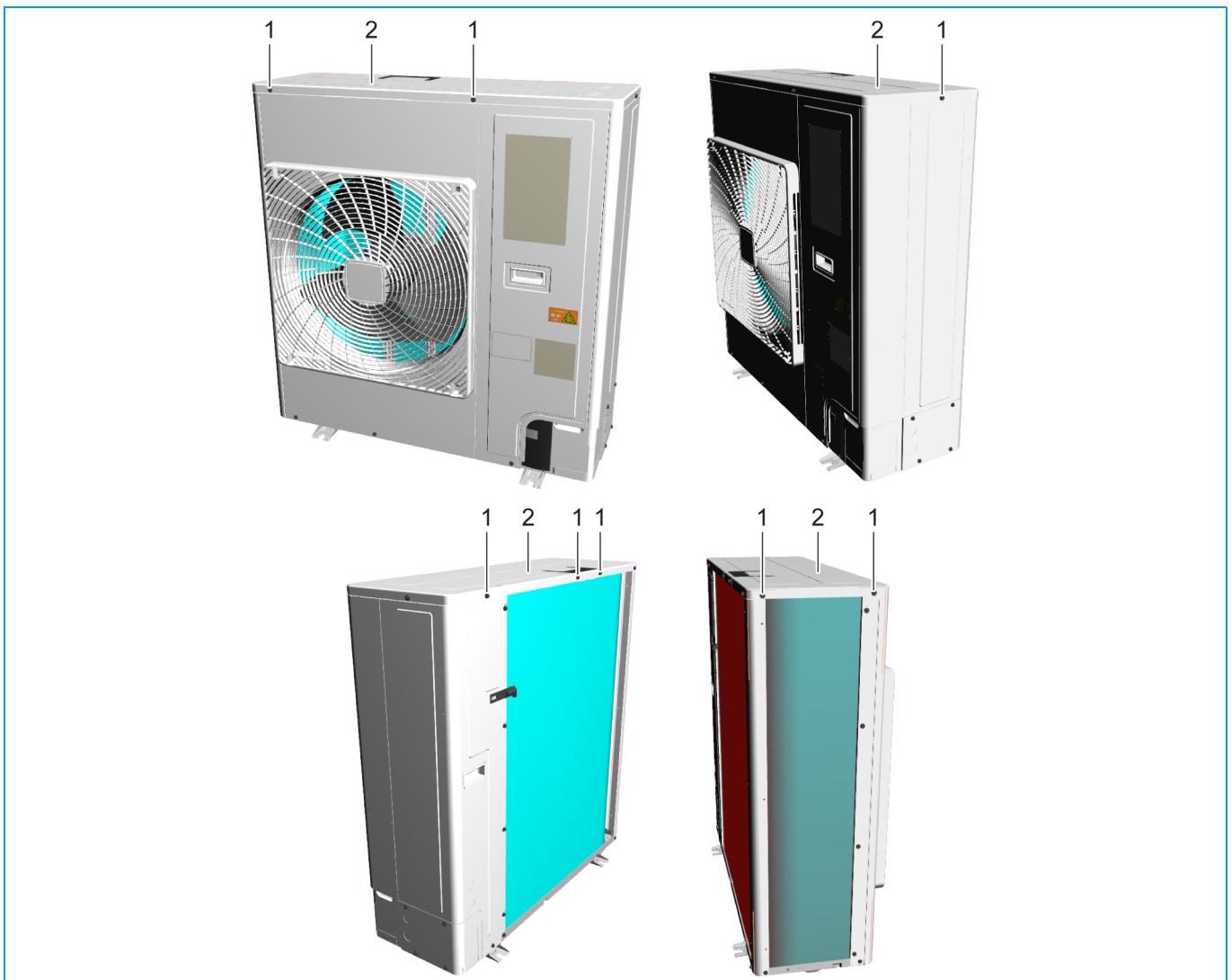
Figure 3-3: Removing the top plate assembly
