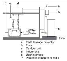
In places with weak reception, keep distances of 3 m or more to avoid electromagnetic disturbance of other equipment and use conduit tubes for power and transmission lines.
