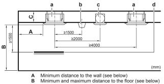
С ≥298 mm: In case of installation with standard decoration panel ≥348 mm: In case of installation with fresh air intake kit
