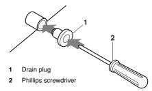
Set the plug and push it by using a Phillips screwdriver
