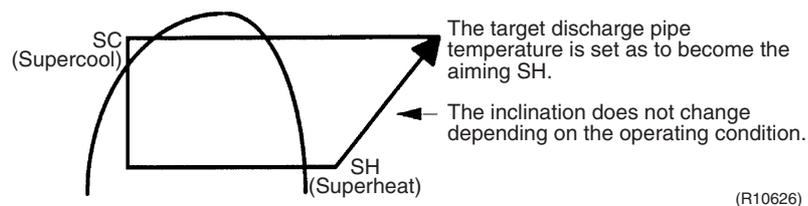
The electronic expansion valve opening and the target discharge pipe temperature are adjusted every 20 seconds. The target discharge pipe temperature is controlled by indoor heat exchanger temperature and outdoor heat exchanger temperature. The opening degree of the electronic expansion valve is controlled by followings.
