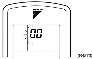
2. Press the TEMP▲ or ▼ button and change the figure until you hear the sound of “beep” or “pi pi”.
