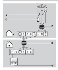
Simultaneous operation system. 1 user interface controls 2 indoor units (indoor units operate simultaneously)
