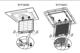
3 Clean the air filter. Use a vacuum cleaner or wash with water. If the air filter is very dirty, use a soft brush and neutral detergent.
