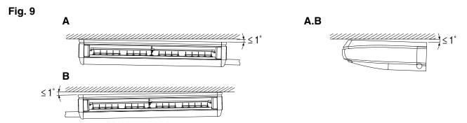
A. When the drain piping is tilted to the right, or to the right and back.
