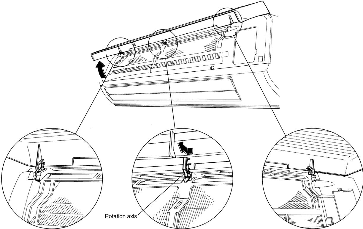
Slide the center rotary axis the left and remove it out.
