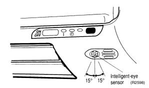
Gently push and slide the sensor to adjust the angle. Aim so that the sensor is pointing to the center of the room, or to the part of the room that is most frequently used.
