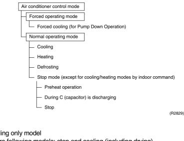
2. For cooling only model There are following models; stop and cooling (including drying).
