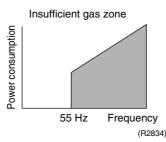
With the conventional function, a power consumption is weak comparing with that in the normal operation when gas is insufficient, and gas insufficiency is detected by checking a power consumption.
