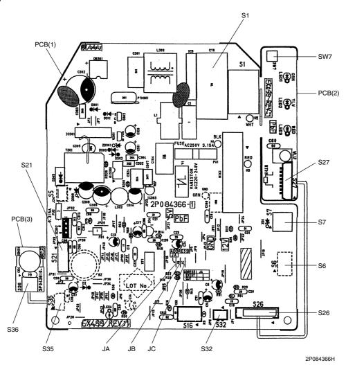
Printed Circuit Board Connector Wiring Diagram
