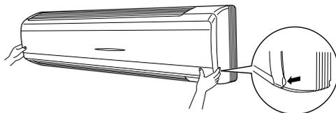
3. **Take off the Titanium Apatite Photocatalytic Air-Purifying Filter.**
