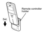
• To remove, pull it upwards.
