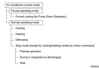
For cooling only model There are following models; stop and cooling (including drying).
