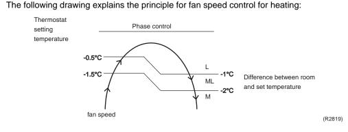
Automatic Air Flow Control for Cooling The following drawing explains the principle of fan speed control for cooling: fan speed  $+1.5^{\circ}C$   $+0.5^{\circ}C$   $+0.5^{\circ}C$ The following drawing explains the principle of fan speed control for cooling: fan speed M  $+2^{\circ}C$ L  $+1^{\circ}C$  M  $+1^{\circ}C$  $+1^{\circ}C$
