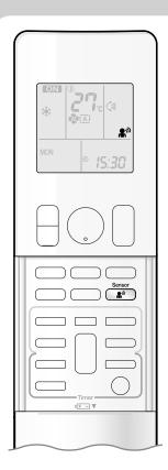
"INTELLIGENT EYE" is the infrared sensor which detects the human movement. If no one is in the room for more than 20 minutes, the operation automatically changes to energy saving operation.
