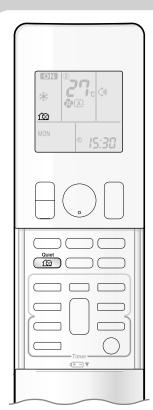
OUTDOOR UNIT QUIET operation lowers the noise level of the outdoor unit by changing the frequency and fan speed on the outdoor unit. This function is convenient during the night.
