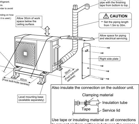
Use tape or insulating material on all connections to prevent air from getting in between the copper piping and the insulation tube.
