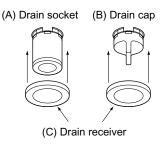
3) Connect vinyl hose on the market (internal diameter of 25 mm) to drain socket (A) (If the house is too long and hangs down, fix it carefully to prevent the kinks.)
