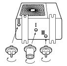
(Be sure not to insert them into wrong drain holes, or there causes water leakage.)
