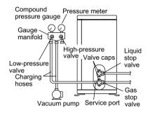
1) Connect projection side of charging hose (which comes from gauge manifold) to gas stop valve's service port.
