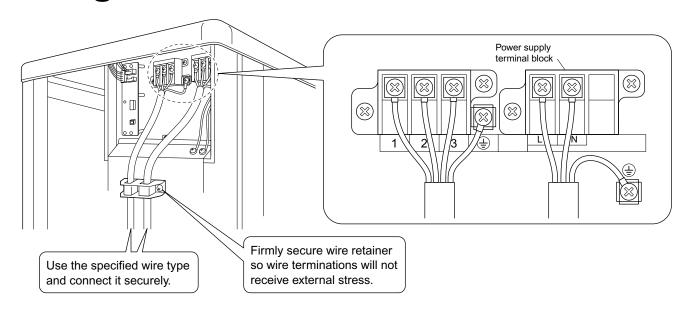
Observe the notes mentioned following when wiring to the power supply terminal board.
