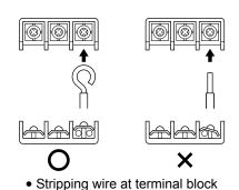
3) Pull the wire and make sure that it does not disconnect. Then fix the wire in place with a wire stop.
