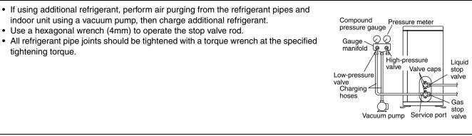
1) Connect projection side of charging hose (which comes from gauge manifold) to gas stop valve's service port.
