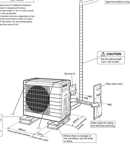
In sites with poor drainage, use block bases for outdoor unit Adjust foot height until the
