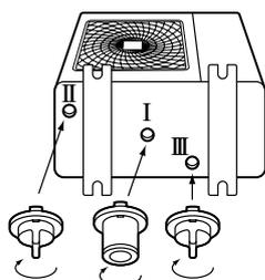
(Be sure not to insert them into wrong drain holes, or there causes water leakage.)
