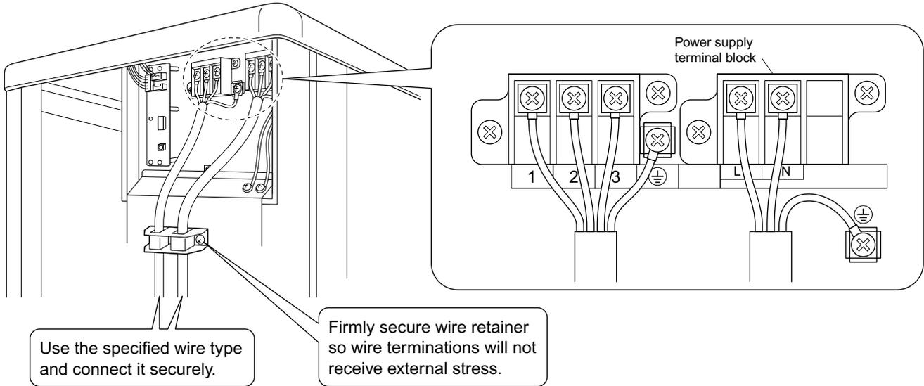
Observe the notes mentioned following when wiring to the power supply terminal board.
