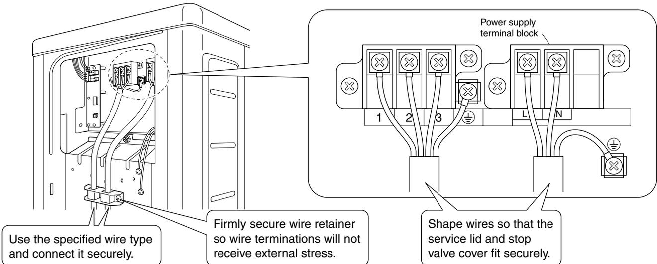
Observe the notes mentioned following when wiring to the power supply terminal board.
