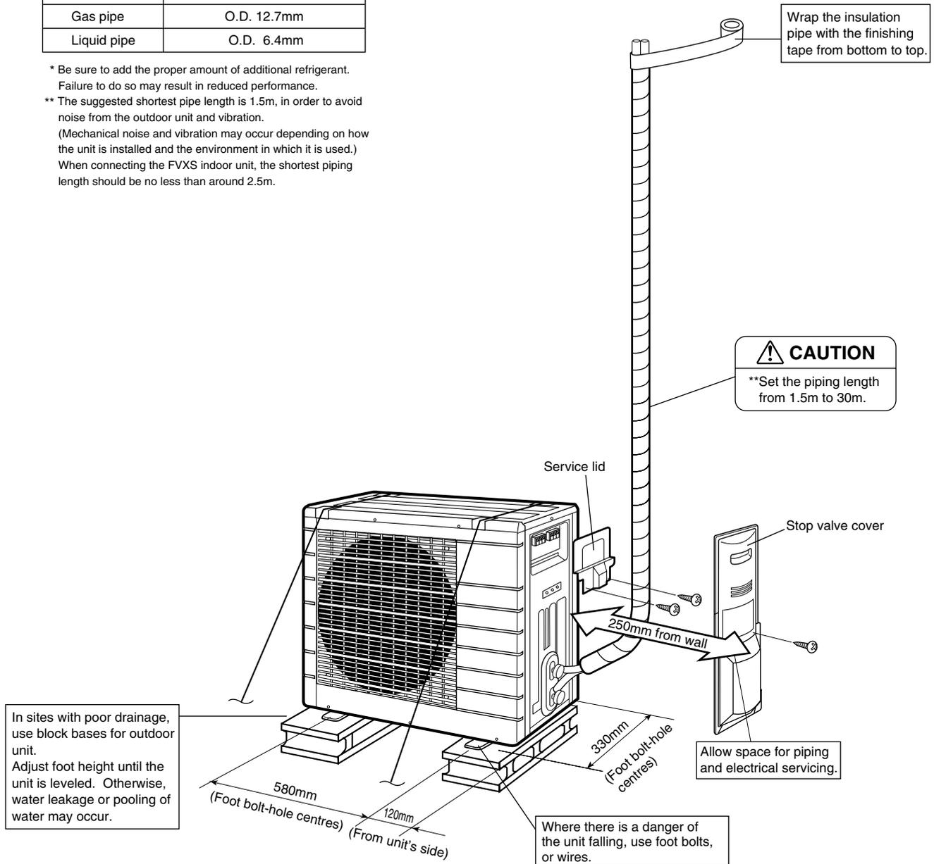
In sites with poor drainage, use block bases for outdoor unit. Adjust foot height until the unit is leveled. Otherwise, water leakage or pooling of water may occur.
