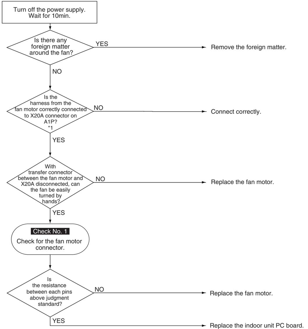
\*1 When there is a relay connector between the connector (X20A) on the indoor PC board and the fan motor, check if the relay connector is correctly connected.
