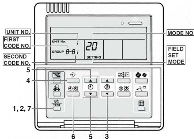
1. When in the normal mode, press the “
