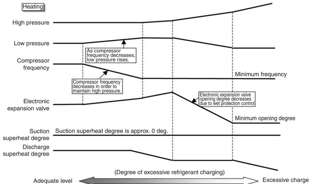
**Check No. 10      Check for factors causing wet operation**
