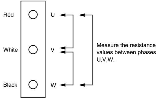
**Check on connector of fan motor (Signal line)**
