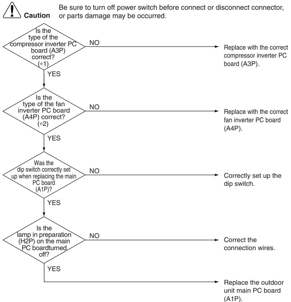
\*1. The types of compressor inverter PC board
