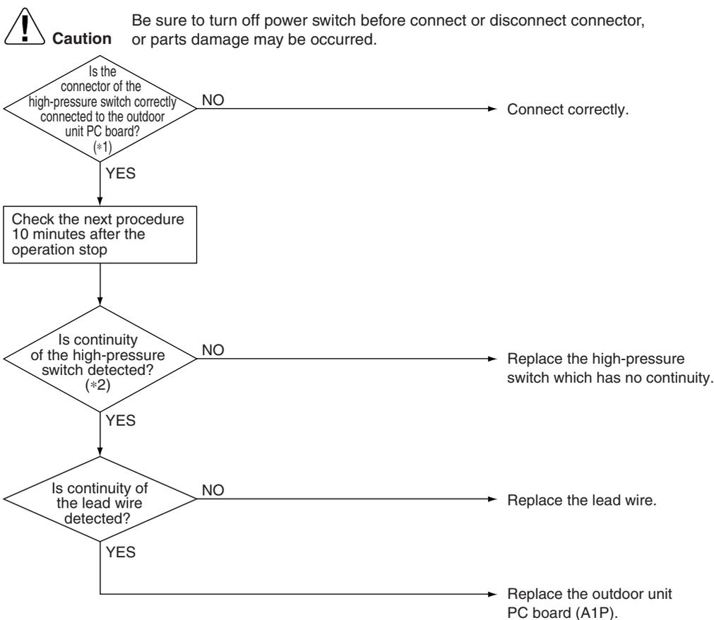
\*1. The connector No. of the high-pressure switch (protection from high-pressure) is shown in the following table.
