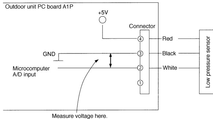
\*2: "Pressure Sensor", pressure/voltage characteristics table.
