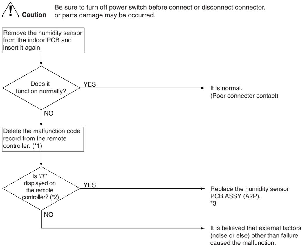
\*1: To delete the record, the **ON/OFF** button of the remote controller must be pushed and held for 5 seconds in the check mode.
