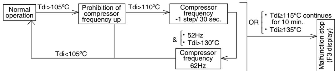
Tdi: Inverter compressor discharge pipe temperature (°C)
