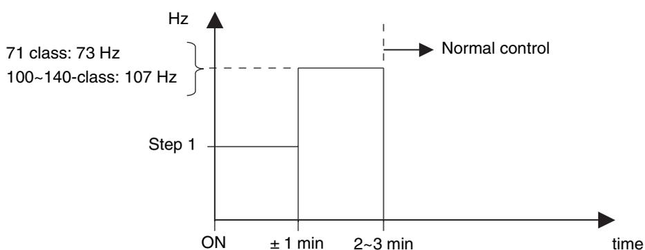
**Ending condition** The starting control will be terminated when the low pressure value < 6 bar or when the maximum starting time of 10 minutes has been reached in case the low pressure value stays > 6 bar.
