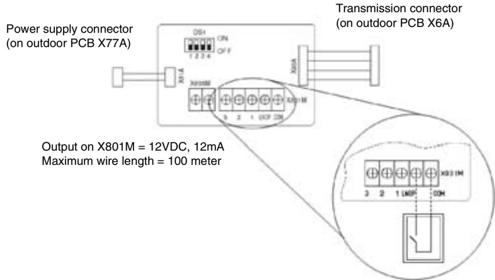
Silent operation will start when the contact on LNOP-COM is closed and will remain active as long as the contact is closed. No field setting on the outdoor unit or by remote controller is required. Silent operation will be ended when the contact is re-opened. Use of the KRP58M enables the use of an external time clock.
