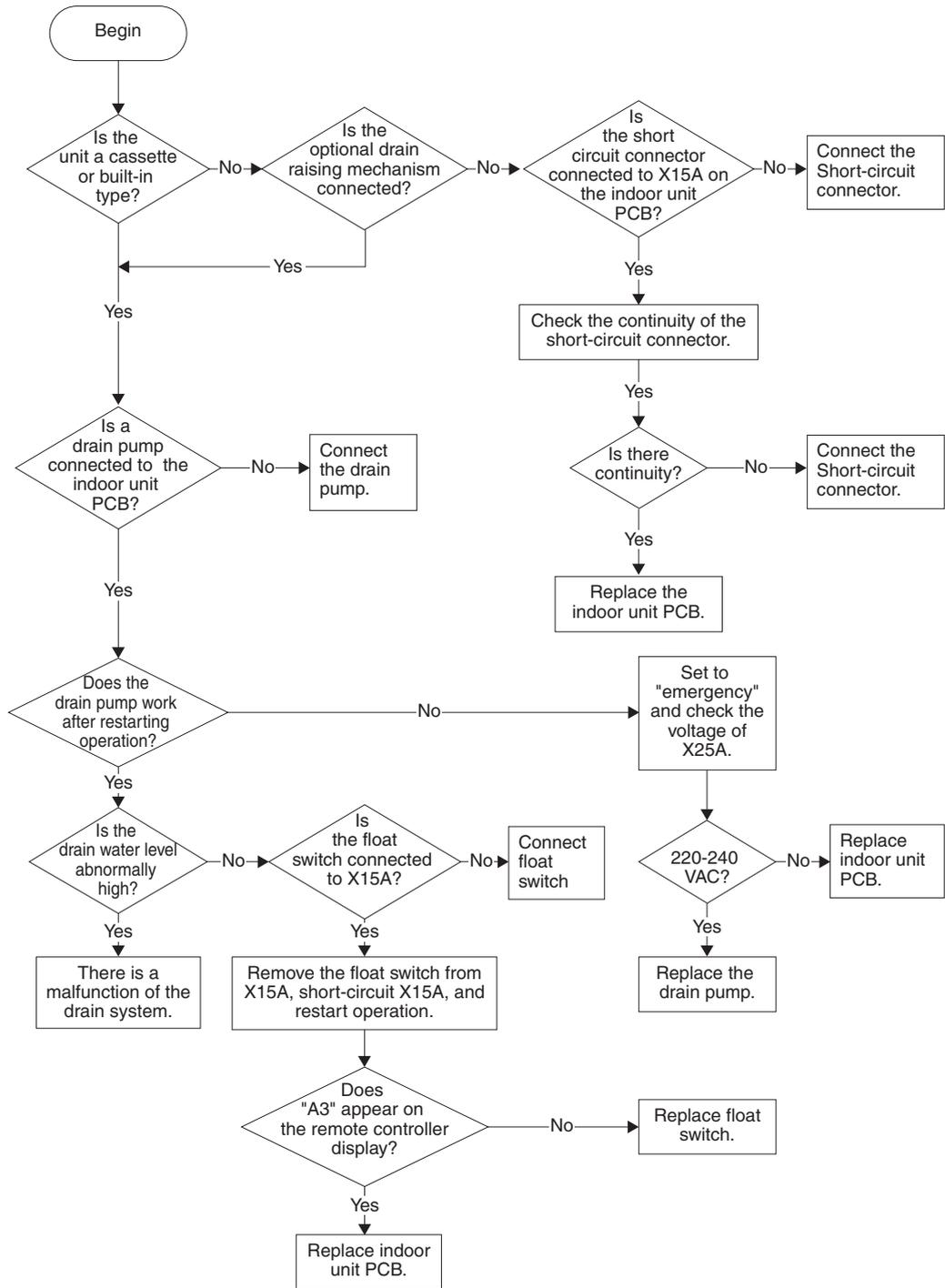
**Remark** If "A3" is detected by a PC board which is not mounted with X15A, the PC board is defective.
