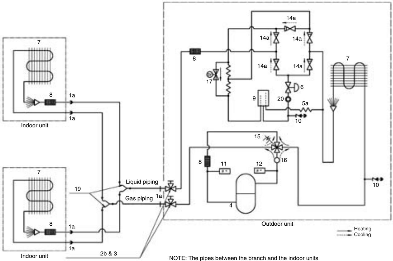
NOTE: The pipes between the branch and the indoor units should have the same size as the indoor connections.
