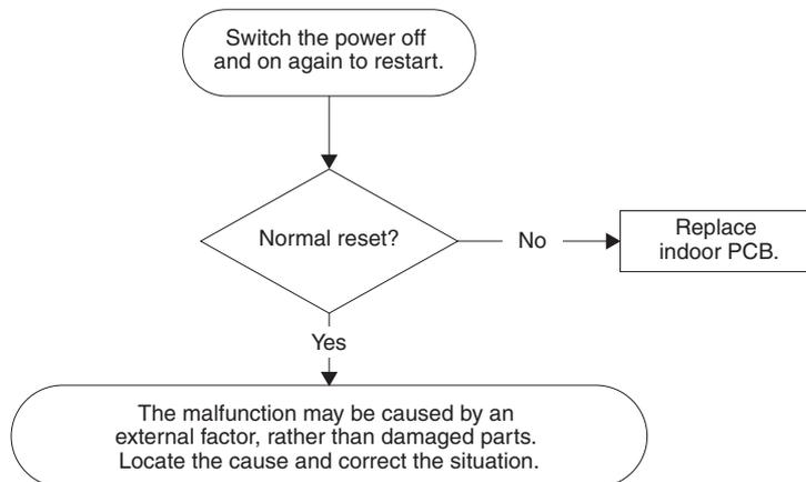
**Caution** Be sure to turn off power switch before connect or disconnect connector, or parts damage may be occurred.
