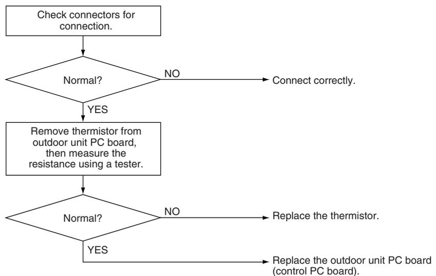
H9 : Malfunction of outdoor temperature thermistor system
