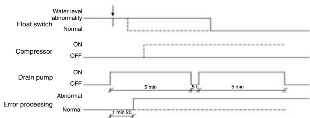
**Float switch activation during thermostat ON**
