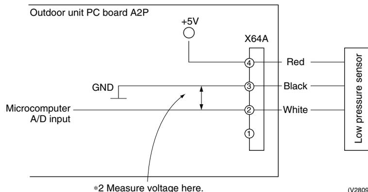
\*2: Refer to pressure sensor, pressure/voltage characteristics table on page 3-115.
