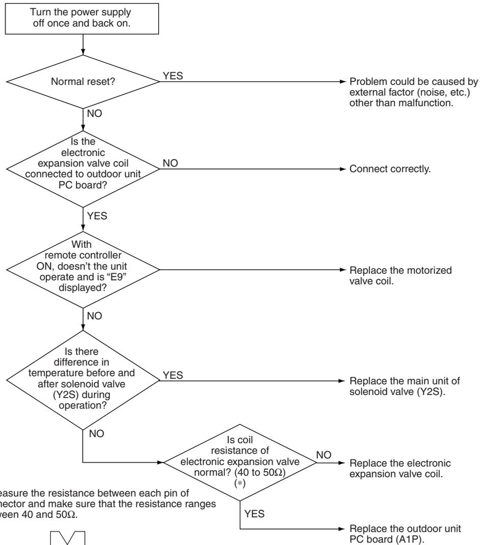
\* Measure the resistance between each pin of connector and make sure that the resistance ranges between 40 and 50Ω.
