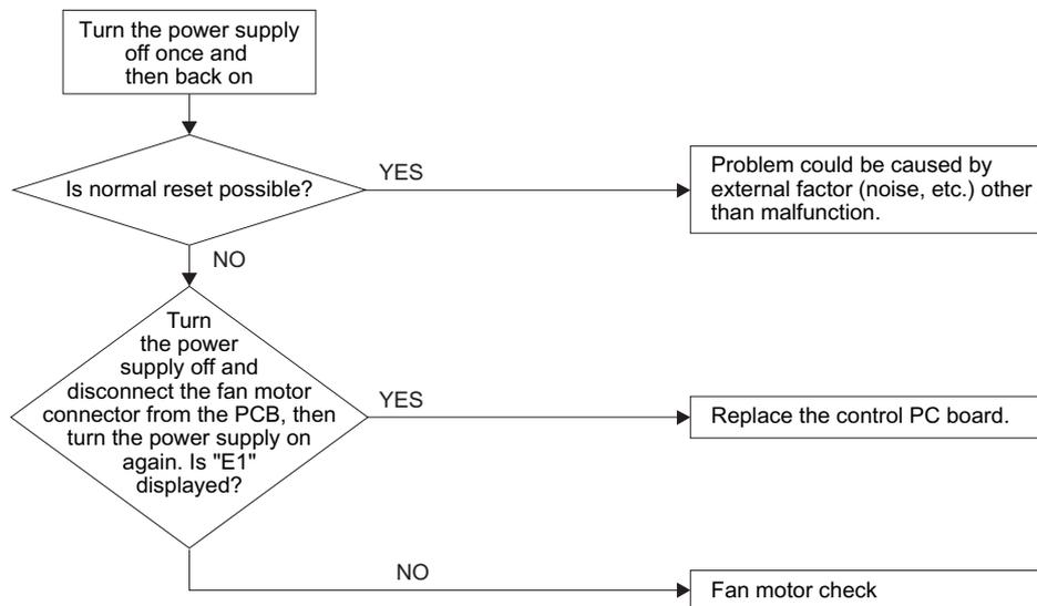
**Caution** Be sure to turn off power switch before connect or disconnect connector, or parts damage may be occurred.
