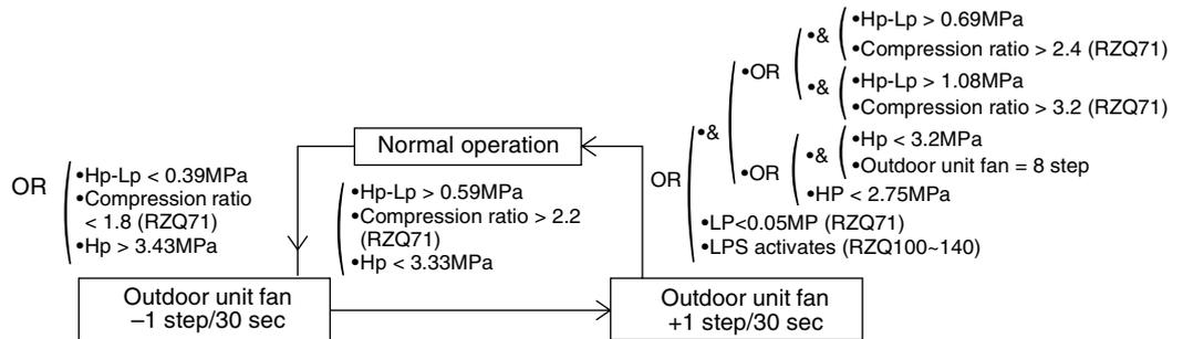
Only the fan speed will be adapted in heating overload conditions. No adjustments to the compressor frequency will be made.
