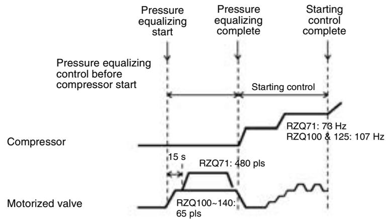
**Expansion valve opening during pressure equalization**
