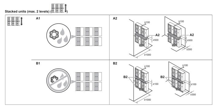
A1=>A2 (A1) If there is danger of drainage dripping and freezing between the upper and lower units... (A2) Then install a roof between the upper and lower units. Install the upper unit high enough above the lower unit to prevent ice buildup at the upper unit's bottom plate. (B1) If there is no danger of drainage dripping and freezing between the upper and lower units...
