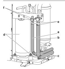
6 If the outdoor unit is installed above the indoor unit, cover the stop valves (f, see above) with sealing material to prevent condensed water on the stop valves from moving to the indoor unit.
