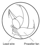
Cautions in mounting the motor Be sure to fix the motor lead wire with a clamp. Not heeding this caution will cause the entanglement of the lead wire around the fan, which will result in damage to the fan.
