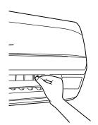
Stop the horizontal flaps at a position where you can hold the tabs and adjust it left and right.
