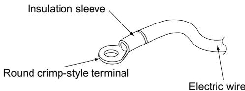
Connect wires of the same gauge to both sides.
