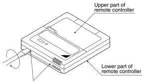
Insert the screwdriver here and gently work off the upper part of remote controller.
