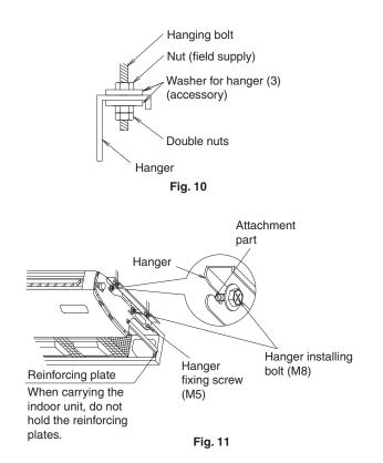
(5) When hanging the indoor unit, make sure to use the level to have better drainage and install it horizontally. Also, if it is possible at the installation site, install so that the drain piping side is slightly lower. (Refer to Fig. 12)
