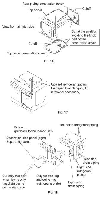
• After piping is finished, cut the removed penetration cover along the shape of piping, and install.
