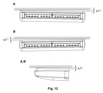
A. When the drain piping is tilted to the right, or to the right and back.
